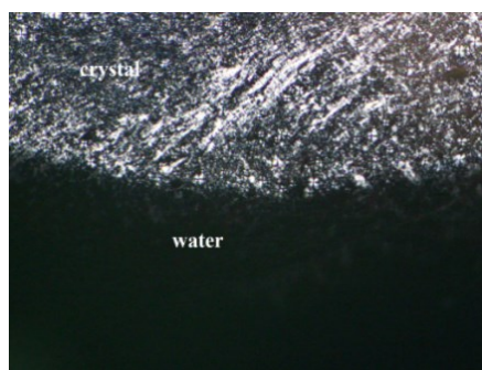
Figure 4. Contact penetration of water into GalPKO at room temperature under x10 magnification
